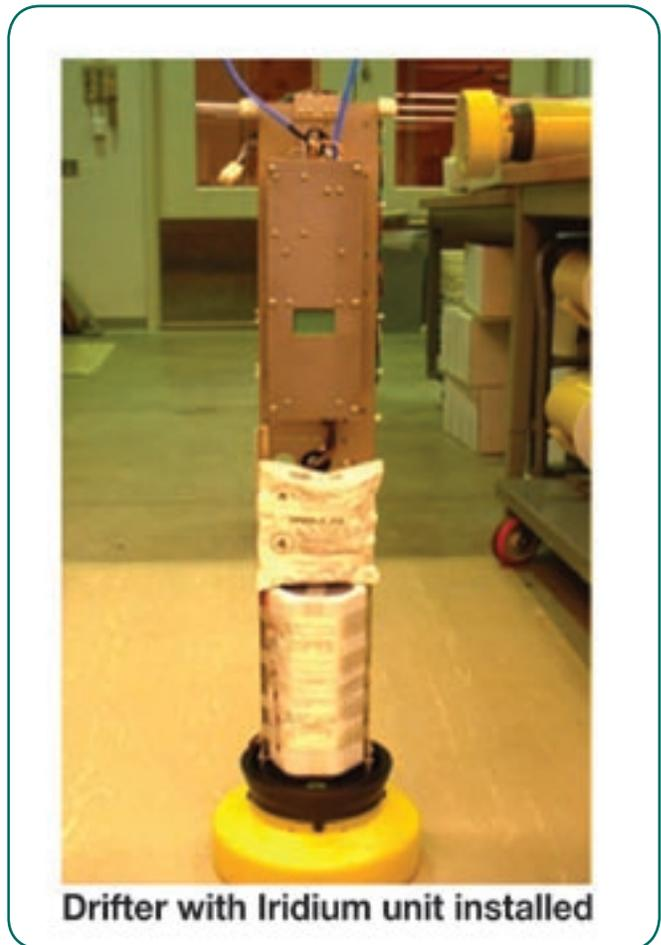
**Drifter with Iridium unit installed**
