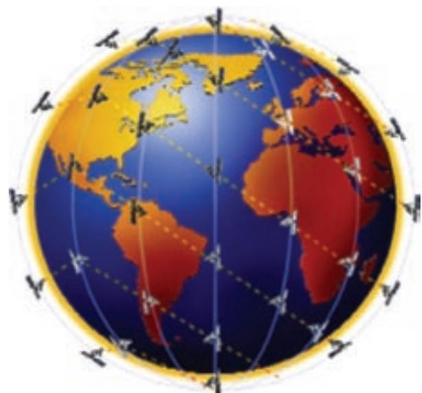
The Iridium constellation consists of 66 operational satellites and 13 spares orbiting in a constellation of six polar planes. Each satellite is cross-linked to four other satellites: two satellites in the same orbital plane and two in an adjacent plane.
